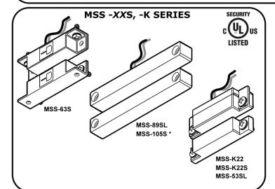
**Specifications** Max Current: 0.25 A Resistive Max Voltage: 30 VDC Max Power: .25 W Resistive The Magnasphere MSS-Concealed series is intended to be connected to a UL Listed compatible control panel for US applications and a ULC Listed compatible control panel for
