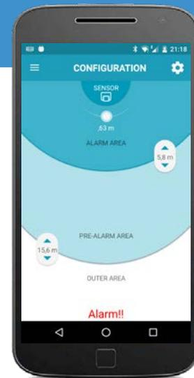
Inxpect's motion processing engines give installers full flexibility with setting alarm and pre-alarm ranges of up to 20m/66ft with an accuracy of 30cm/1ft, sensitivity, and how alarm, pre-alarm, tamper and fault signals are signaled to the panel. Forget about cords, dip switches or faulty potentiometers: with the free Inxpect mobile app for Android and iOS, configuring MSK sensors is easy and straightforward.
