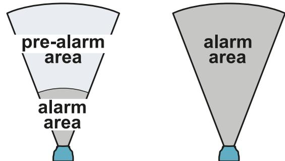
Motion in the alarm area triggers an alarm, motion in the pre-alarm area triggers a pre-alarm.
