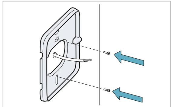
2. Fasten the bracket to the plate, passing the Ethernet cable into the bracket.
