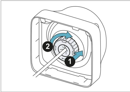
**NOTICE:** if it is necessary to unscrew the ferrule, to prevent damaging the closure mechanism, press and then turn the ferrule in a counter-clockwise direction.
