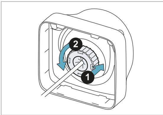
10. Fasten the sensor case to the plate.
