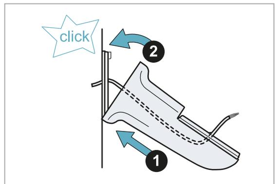
3. Insert the ferrule, the cable protection ring and the cable protector in the cable and insert the RJ45 connector into the Ethernet port, see steps 2–9 of the "Assemble the sensor" on the previous page procedure.
