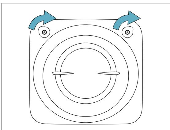
2. Fasten the case of the sensor to the plate using the provided screw.
