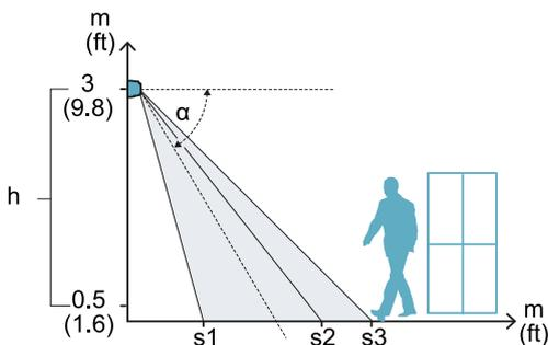
The actual field of vision of the sensor (detection start and end,  $s_1$  and  $s_2$ ) depends on:
