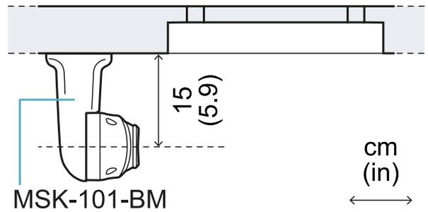
Example of installation with MSK-101-BM bracket.
