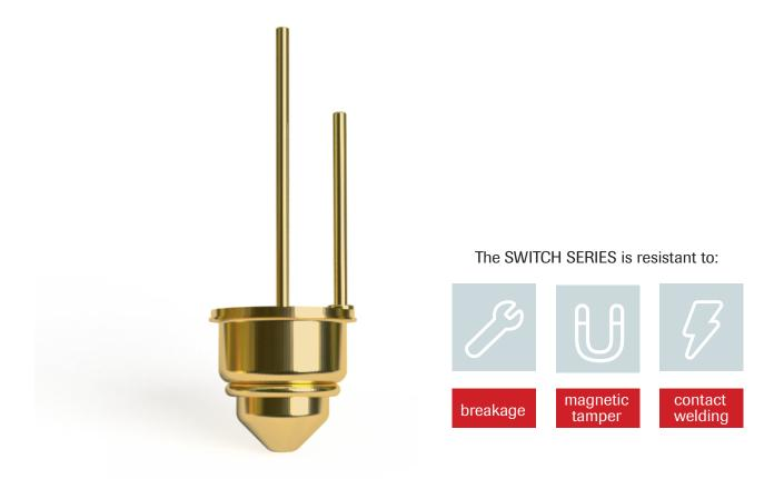
The MAGNASPHERE S series is used in the security industry for door and window sensors in Open Loop alarm systems. It has a wider actuation zone in the X or Y axis than other Form B MAGNASPHERE switches. The robust all metal construction is highly resistant to magnetic tamper and defeat, and permanent contact welding from power surges.
