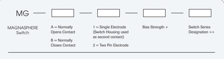
**EXAMPLE** MG-A2-3.0-N = MAGNASPHERE switch, N.O. (Normally Open), Two pin electrode, 3.0 Bias Strength, N Series
