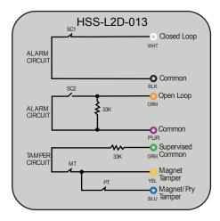
Legend SC = Secure Contact MT = Magnet Tamper PT = Pry Tamper ##K = Resistor 36" [91cm] Armored Cable (Std.), (See Page 41 for Custom Cable Length)
